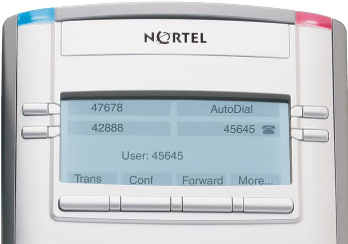
Figure 10 shows an IP Phone 1140E logged in as a Remote phone to an IP Phone 1120E Office phone. Fewer display lines are available on the IP Phone 1120E, so the display provides less information.
