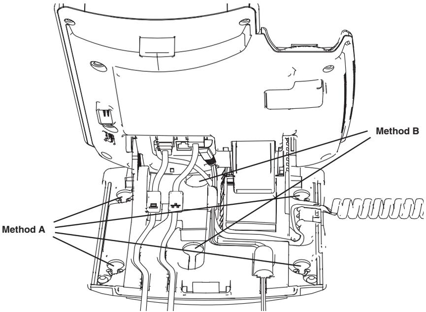
8. Wall-mount your phone (optional). Your IP Phone 1120E can be mounted either by: (Method A) using the mounting holes on the bottom of the phone stand, or (Method B) using a traditional-style wall-mount box with an RJ-45 connector and a 15-cm (6-inch) RJ-45 cord (not provided).
