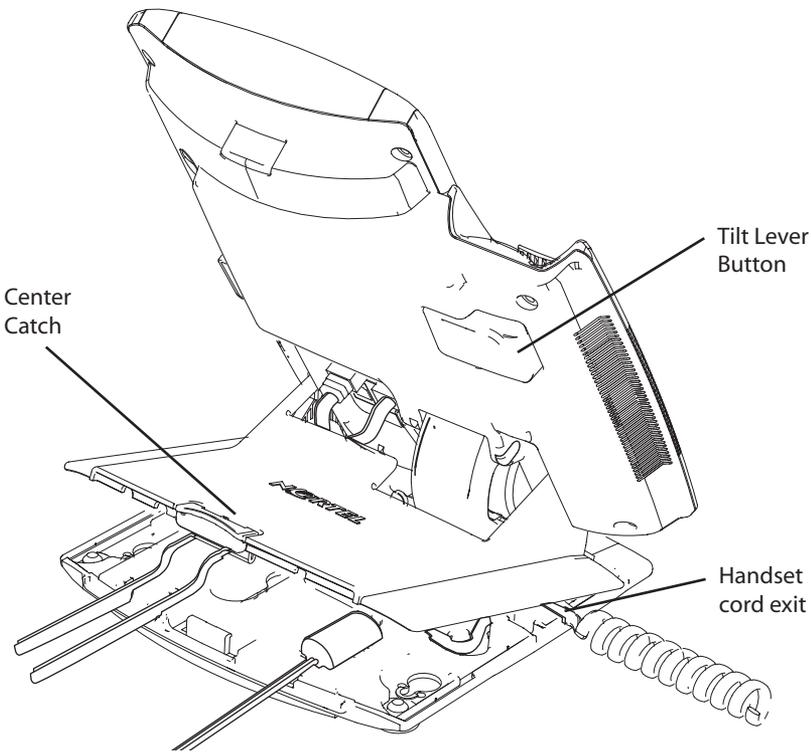
2. Connect the AC power adapter (optional). Connect the adapter to the AC adapter jack in the bottom of the phone. Form a small bend in the cable, and then thread the adapter cord through the channels in the stand.
