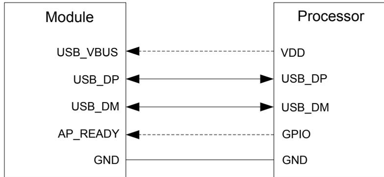
**Figure 4: USB Application with Suspend Function**
