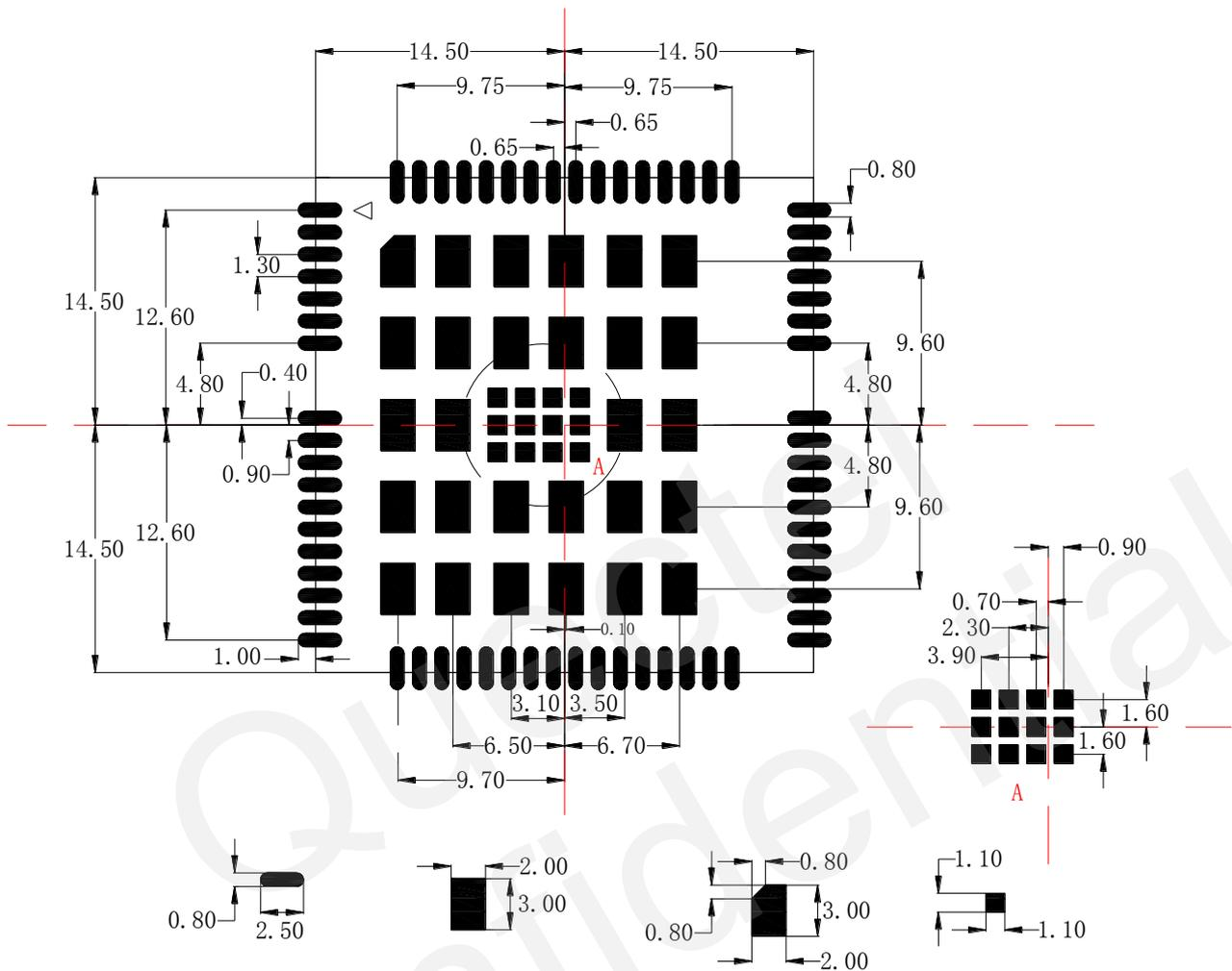
Figure 42: Recommended Footprint (Top View)
