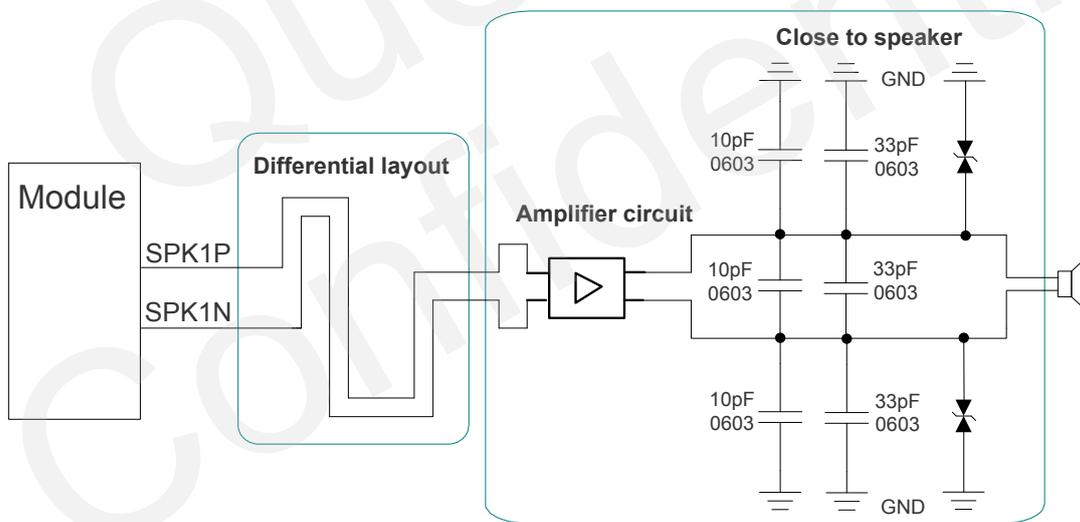
Figure 23: Reference Design with an Amplifier for AOUT1
