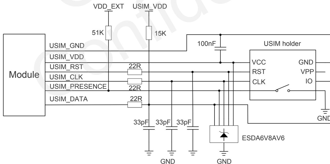
**Figure 27: Reference Circuit of the 8 Pin USIM Card**
