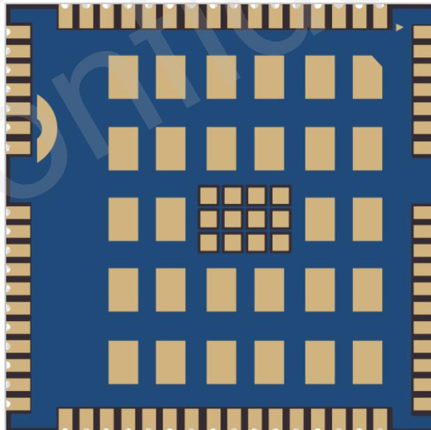
Figure 44: Bottom View of the Module
