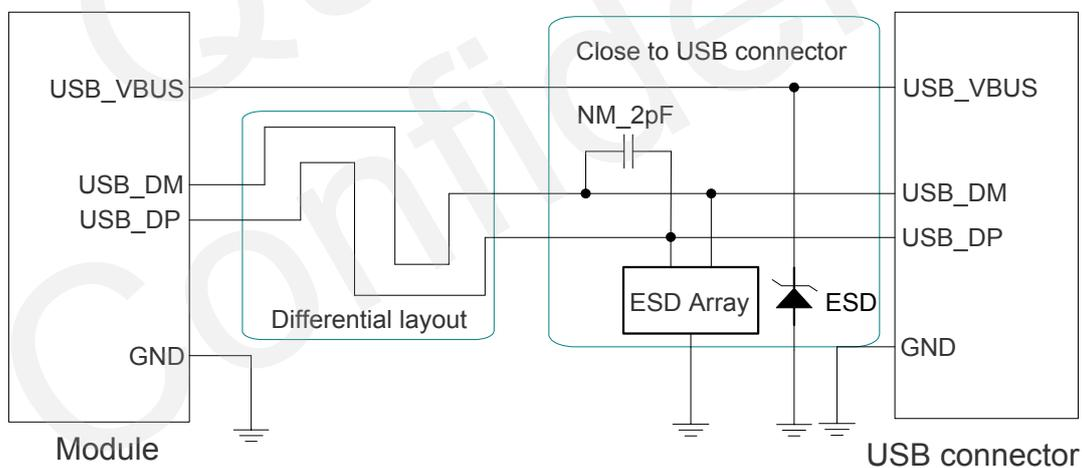
**Figure 31: Reference Circuit of USB Application**
