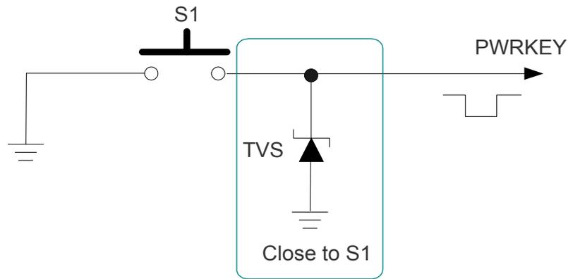
**Figure 9: Turn on the Module by Keystroke**
