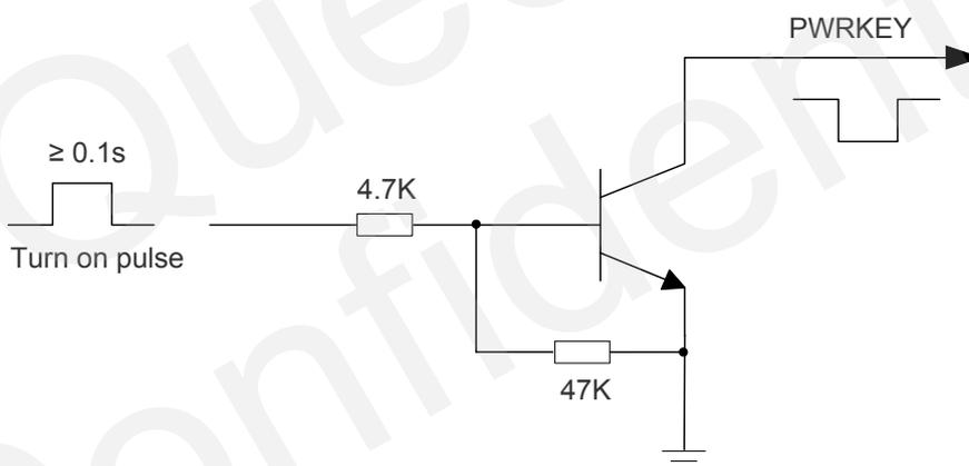
**Figure 8: Turn on the Module by Driving Circuit**
