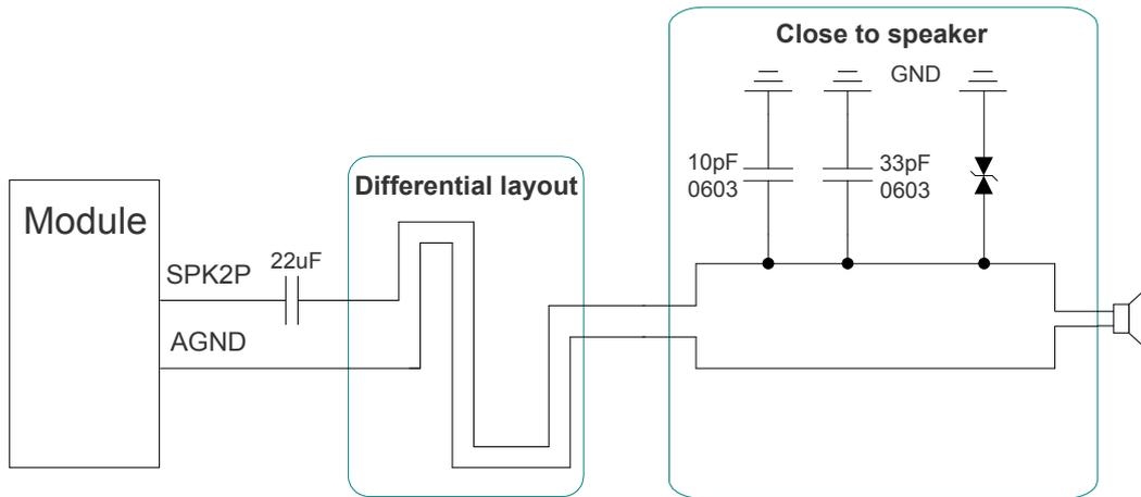
Figure 24: Reference Design for AOUT2
