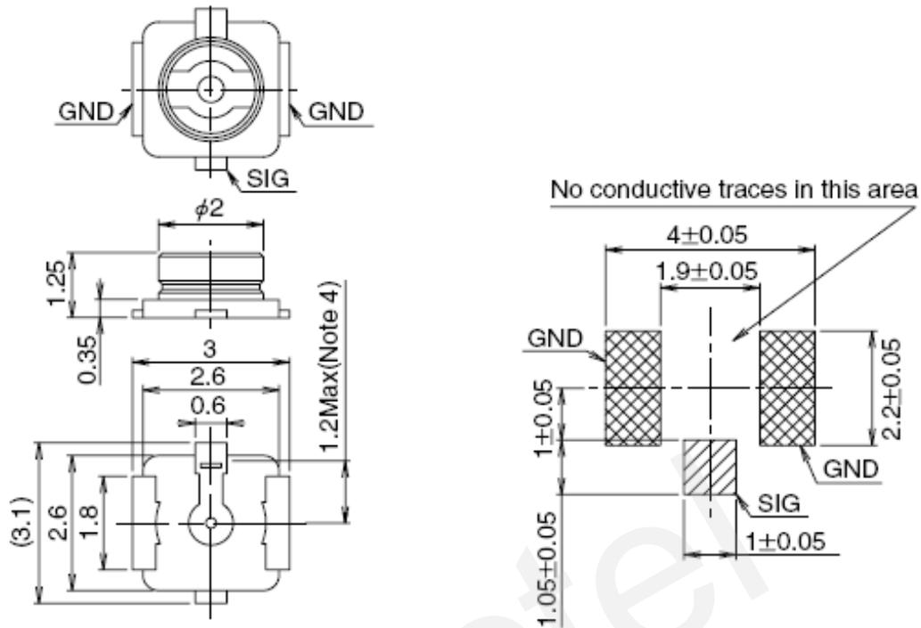
Figure 36: Dimensions of the UF.L-R-SMT Connector (Unit: mm)
