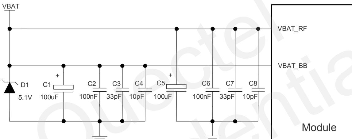
**Figure 6: Star Structure of the Power Supply**
