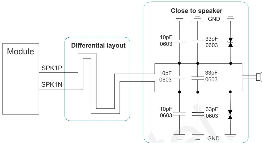
Figure 22: Reference Design for AOUT1
