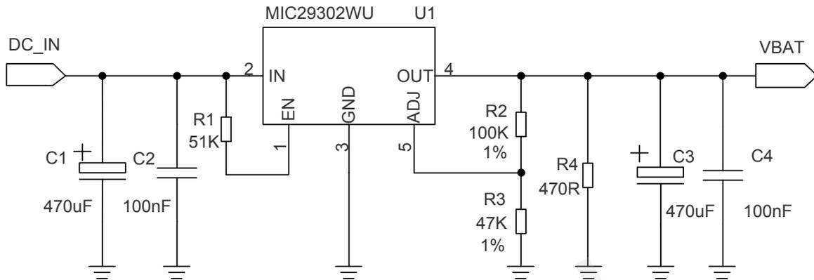
Figure 7: Reference Circuit of Power Supply
