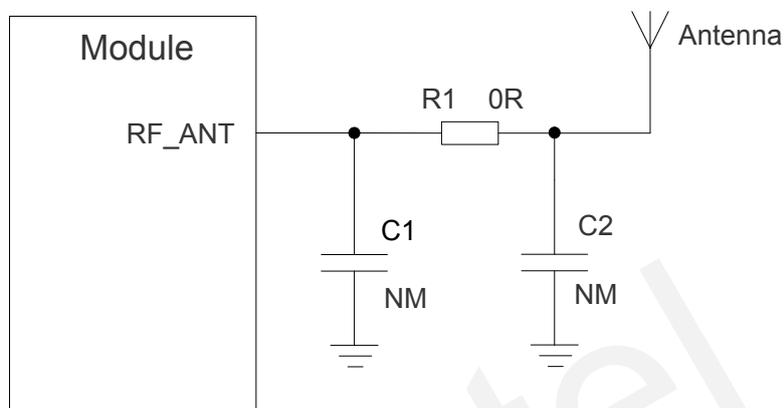
Figure 35: Reference Circuit of Antenna Interface
