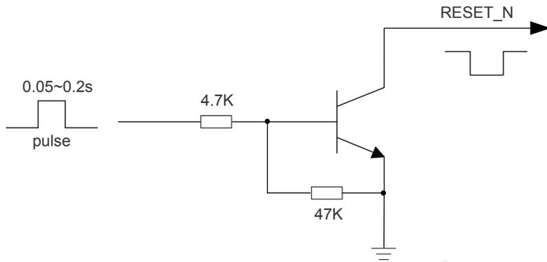
**Figure 12: Reference Circuit of RESET\_N**
