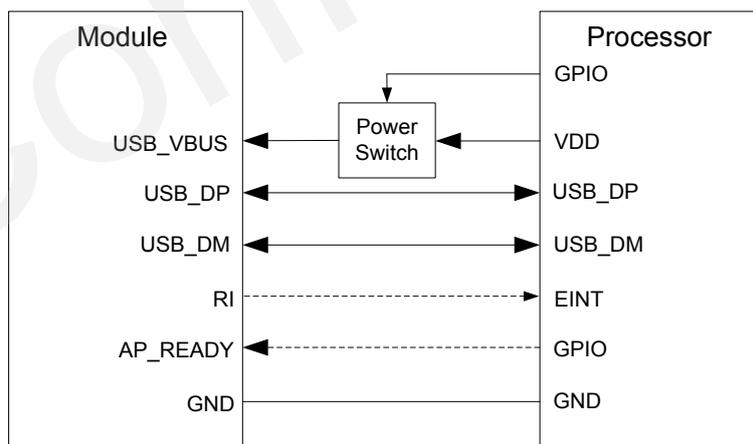
**Figure 5: USB Sleep Application without Suspend Function**
