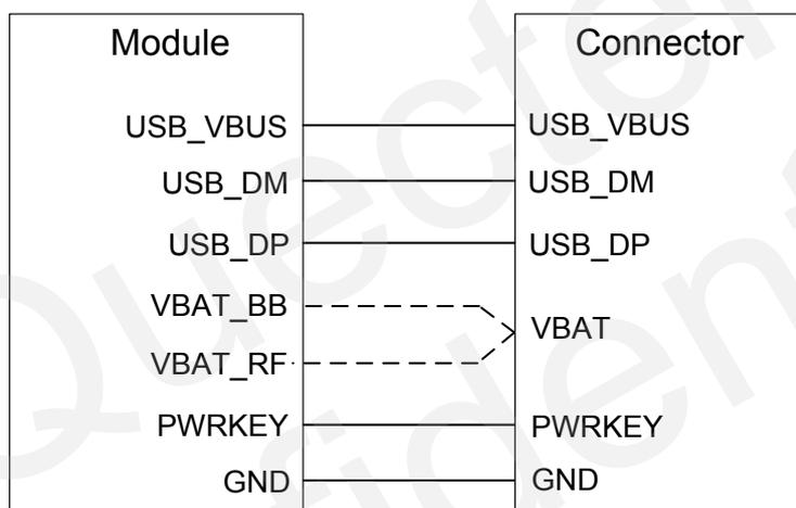
Figure 32: Test Points of Firmware Upgrade
