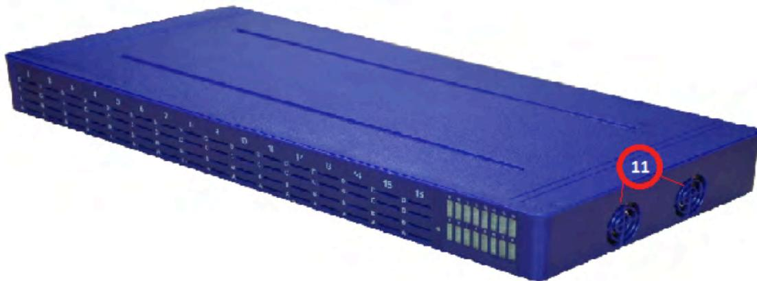
**1**, SIM slots: The 16/64 Madcom device can read 64 SIMs totally. It means the gateway can support 16 calls concurrently (16 channels), and each channel can read 4 SIMs named *A,B,C,D* (This SIMs will rotate to avoid blocking).
